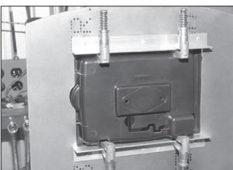
Using at least two Cleco® edge clamps, clip the Panel Dock to the rails. This will allow you to determine how it should look from the front before you drill any holes.
