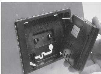
The Panel Dock has been designed to allow the cables that are included with the GPS to be used. We have cut a "keyhole" in the back of the dock to allow the antenna cable to be inserted. These holes have the unique feature of keeping the cables from disappearing behind the panel when the GPS is removed. If desired, you may cover the larger holes using rubber grommets.
