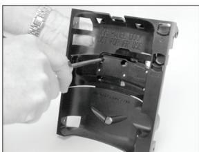
Using the 4 sets of screws and nuts, attach the bracket to the inside of the Panel Dock. Tight securely but *do not overtighten* the screws - it may result in cracking of the bracket.
