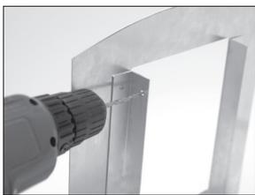
There are a number of ways in which you may choose to drill the holes. You can remove the rails from the panel and drill them on a drill press, or you may use an angle drill to drill them in the plane. Just be careful to make accurate holes at the marks you made, and you will be fine.
