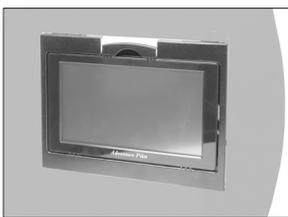
Upon attaching the Battery Power Cable to the GPS, snap the GPS into place in the Panel Dock.
