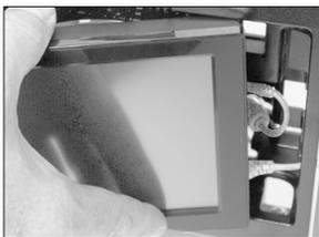
Route the Cable back into the Panel Dock through the opening on the side of the Dock. Plug the Cable into the Power Jack of the GPS, located in the lower part of the unit.
