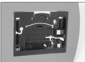
With the Panel Dock secured with the edge clamps you can insert your portable device and verify that it is at the correct depth and that the latching mechanism works properly.
