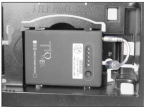
If you wish to power your iFly 700 Series unit from external Battery, then take a Battery Power Cable, which will be attached to the GPS, and route it through the opening, as shown in the photo. Attach one end of the Cable to the Battery jack. Make sure the Battery is inserted and secured (snapped in place) in the designated opening within the Panel Dock.
