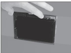
To remove the Garmin 660 slide the release tab to the left and the Garmin 660 will be released and top of the GPS will pop out.
