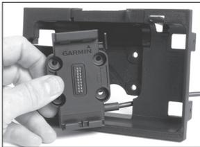
Take the power connector (**yoke mount**) which comes with the aera GPS. You can also purchase a Bare wire connector from Garmin for the aera 660 and install it into the AirGizmos Panel Dock. (Garmin part number #010-12373-01)
