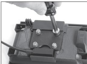
You should remove any rubber spacers in the Garmin connector so that it nests properly in the Panel Dock. Using a remaining hardware (4 screws, nuts, and washers) included in Panel Dock package, securely fasten the power connector.
