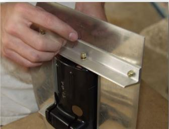
The bolts we provide have an integral washer on the screw-head side. This provides adequate distribution of force on the plastic to keep it from cracking.
