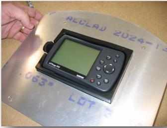
With the Panel Dock secured with the edge clamps you can insert your portable device and verify that it is at the correct depth and that the latching mechanism works properly.
