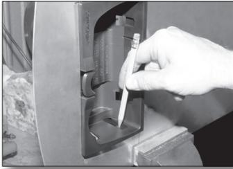
Remove one edge clamp at a time and mark the position of each hole with a pen. Use a circular motion to mark the outer edges of the hole. This will make it easier to determine the exact center.
